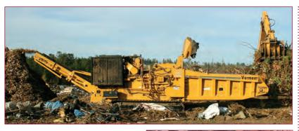
The wood grinding program at the landfill has been very successful. The chips are used as landfill cover and take up much less space than unprocessed materials. Unfortunately, items like propane tanks and scrap metal, right, are sometimes thrown in the yard waste pile. The City encourages residents to be careful, as metal pieces can cause significant damage to the grinding machine, increasing costs to the taxpayers.
