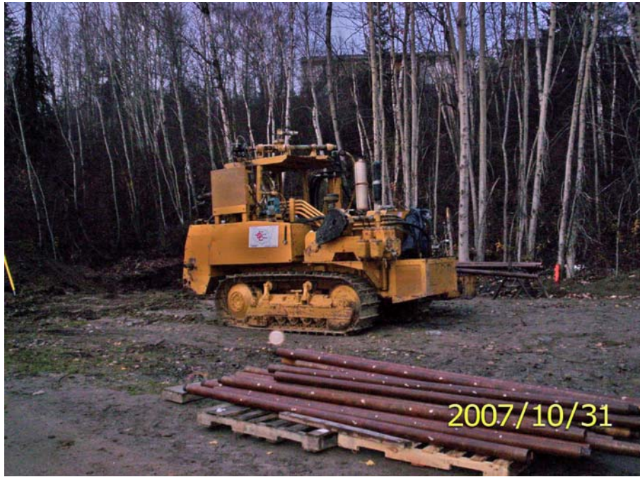
Photo 25: Horizontal drilling rig at HD4.
