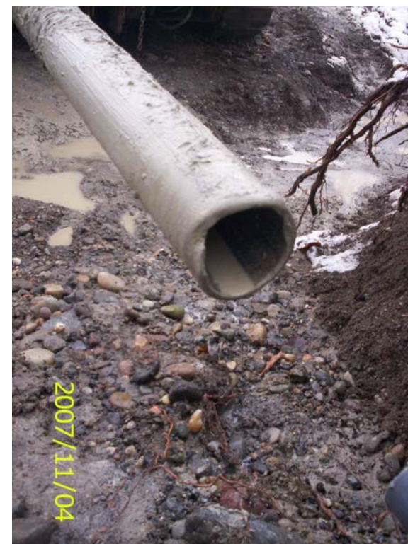
Photo 35: Broken drill rod at HD1.
