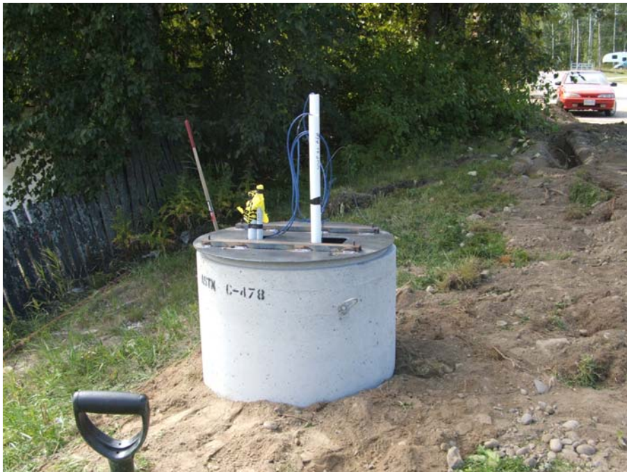
Photo 16: VWP and electrical conduit at BH21.
