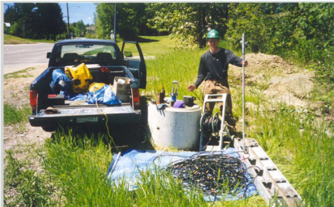
Photo 8: Spiral Probe and 505 foot SI cable ready to be lowered down SI-3 on Abbott Drive
