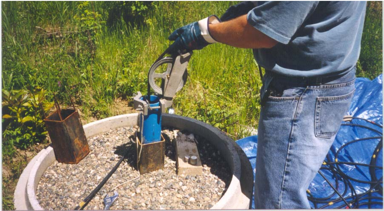
Photo 7: Lowering SI probe down SI pipe at SI-2 location.
