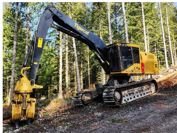
Log loader (hoe-chucker) Tigercat LS 855 E (L01)
