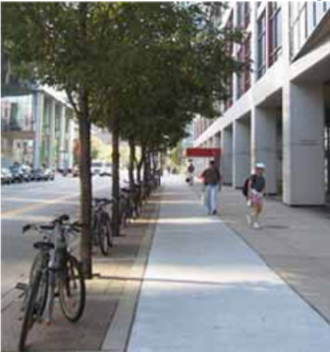
Photo 35: Example where interlocking pavers can be used to differentiate clear path of travel from street element zone and building frontage zone
