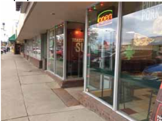
Photo 54: Curb ramps leading into businesses such as Quiznos and Karin's are hard to detect for people who have low vision
