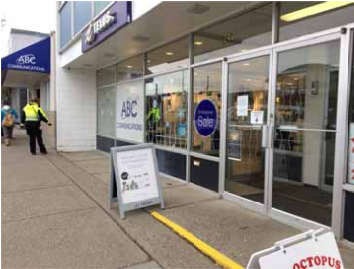
Photo 116: Sandwich boards obstruct the accessible path of travel
