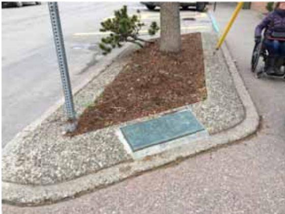
Photo 77: Pebbled planter bed in front of CIBC lacks sufficient colour contrast with surroundings for people with low vision
