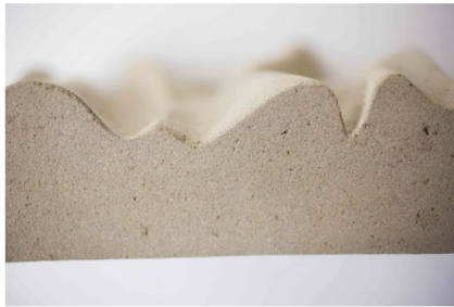
CASTED WOOD – EXPERIMENTS WITH WOOD DUST AND NANO CELLULOSE
