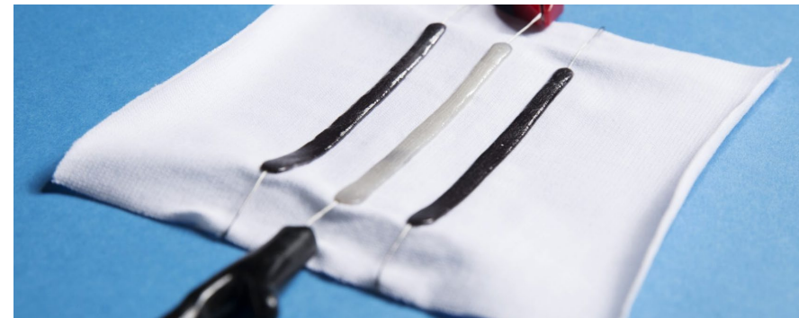
FUNCTIONAL CELLULOSIC STRUCTURES ON FABRICS BY 3D PRINTING
