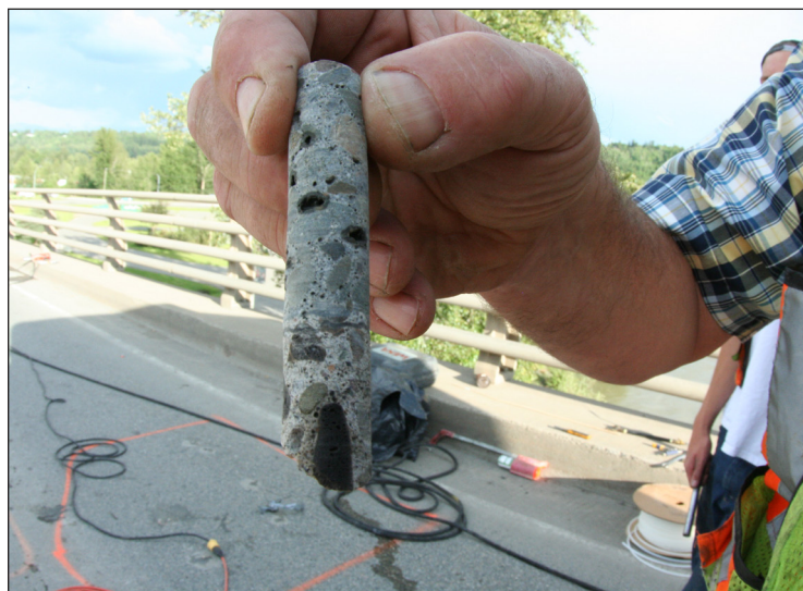
A core sample taken from the Moffat Bridge during repair.
