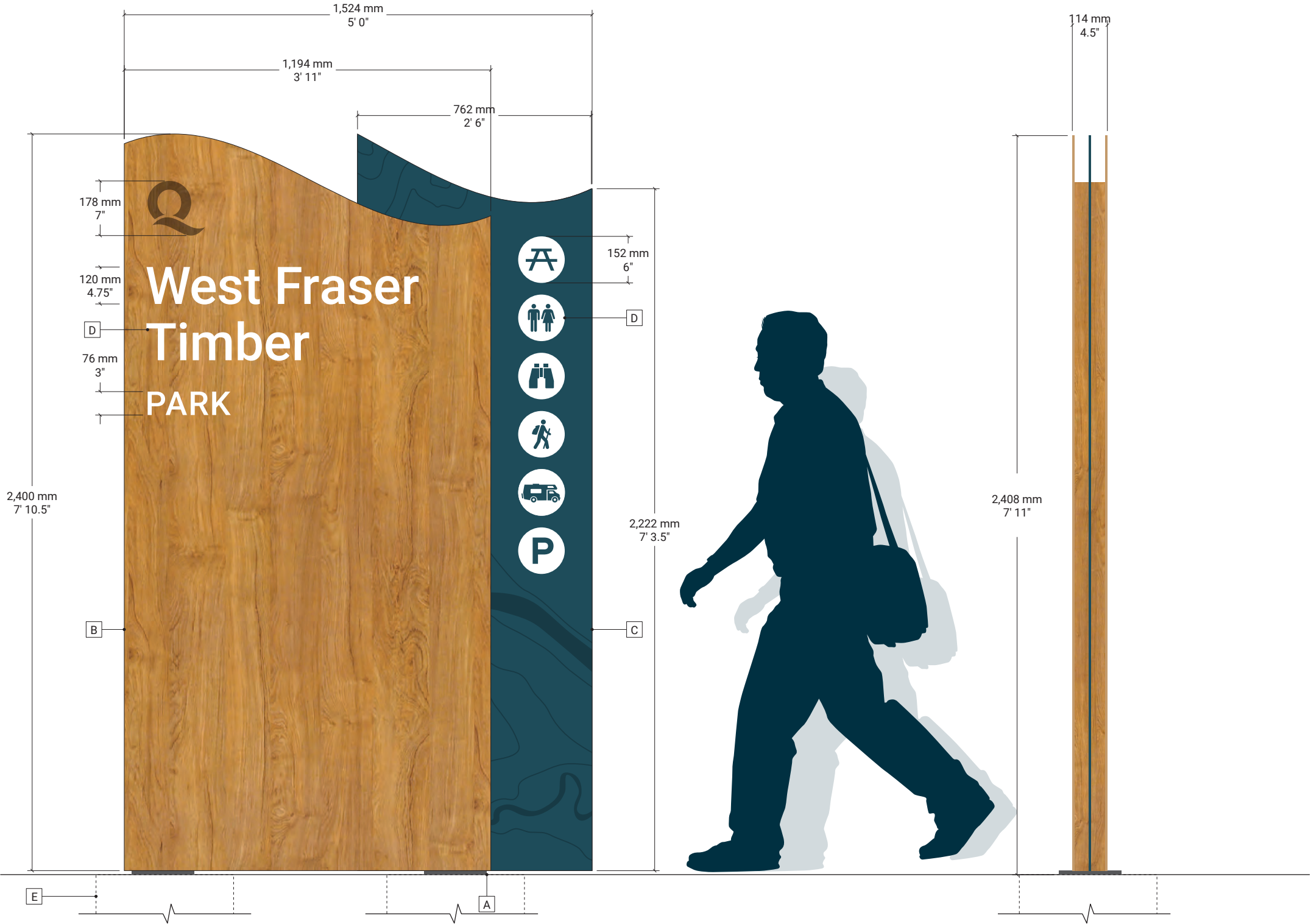
1 Sign Detail - Front View Scale 1:15
