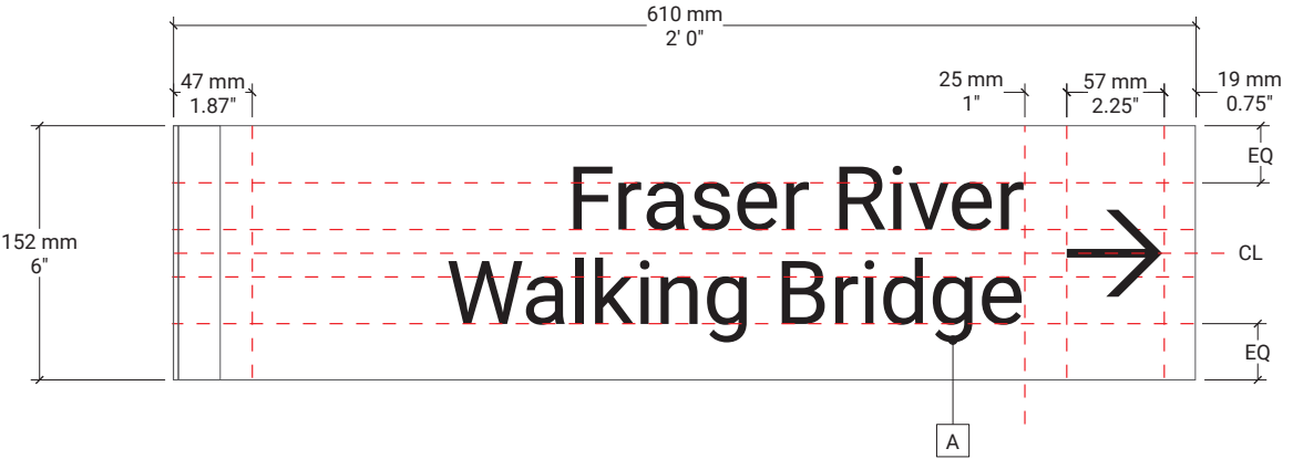
3 Sign Panel Detail - Double Line Destination Scale 1:5
