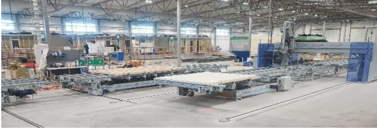
Nailing bridge and modular construction in the background in Sweden (Photo: G. Wimmers)
