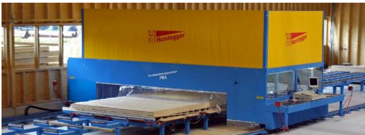
Hundegger PBA is a gantry style cutting machine for solid wood panels (Photo: Hundegger)
