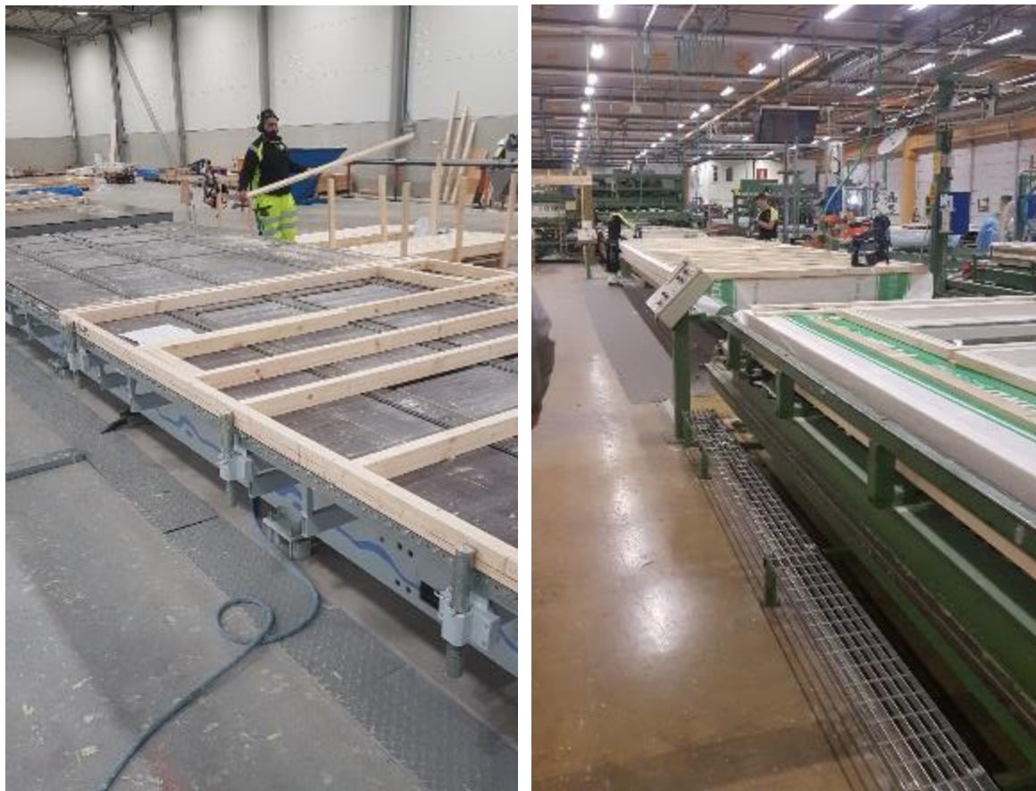
Manufacturing tables from different manufacturers, with clamps in Sweden (Photos: G. Wimmers)
