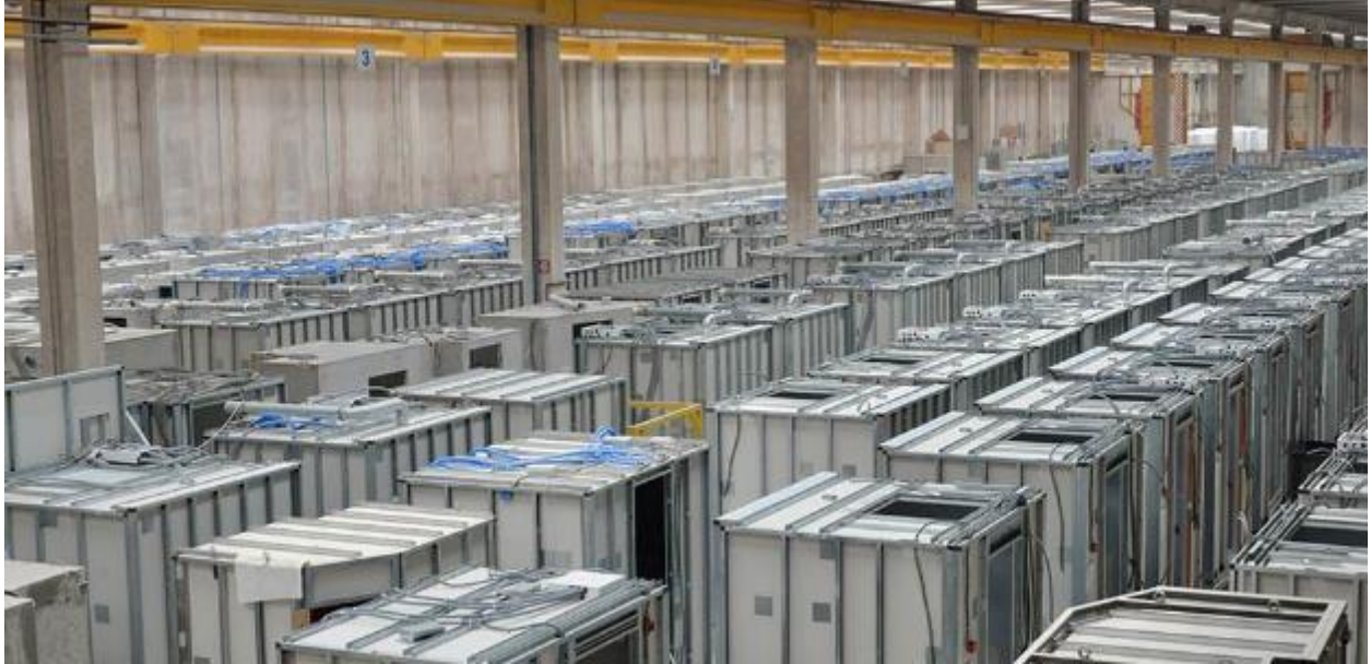
Bathroom Pods premanufactured by specialized company (Photo: Euro Components)
