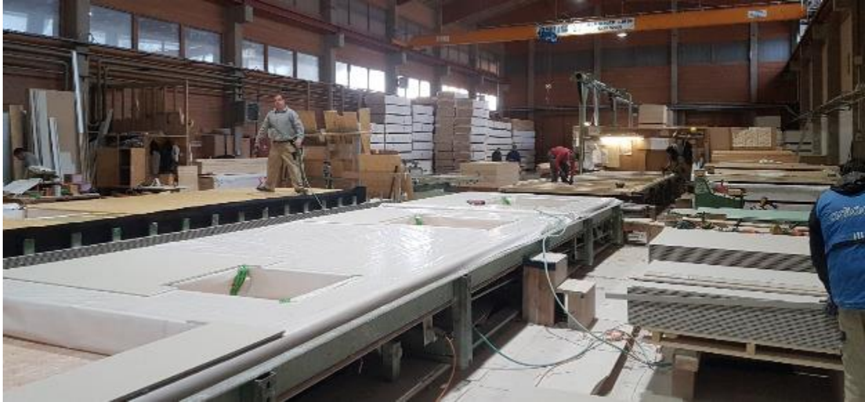
Prefabrication line with large tables and no automation in Austria (Photo: G. Wimmers)
