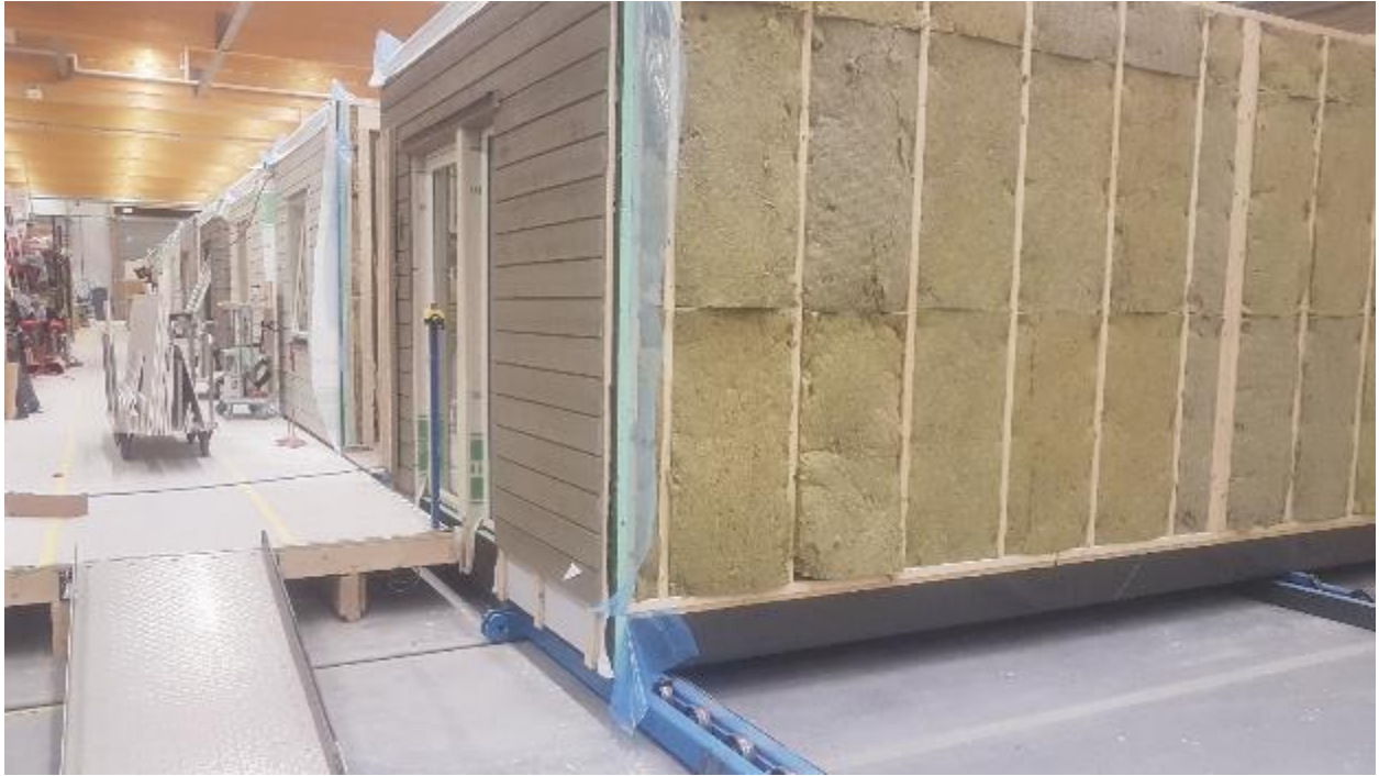
Prefabricated modules showing finished wall and interior connector wall to next module in Sweden (Photo: G. Wimmers)
