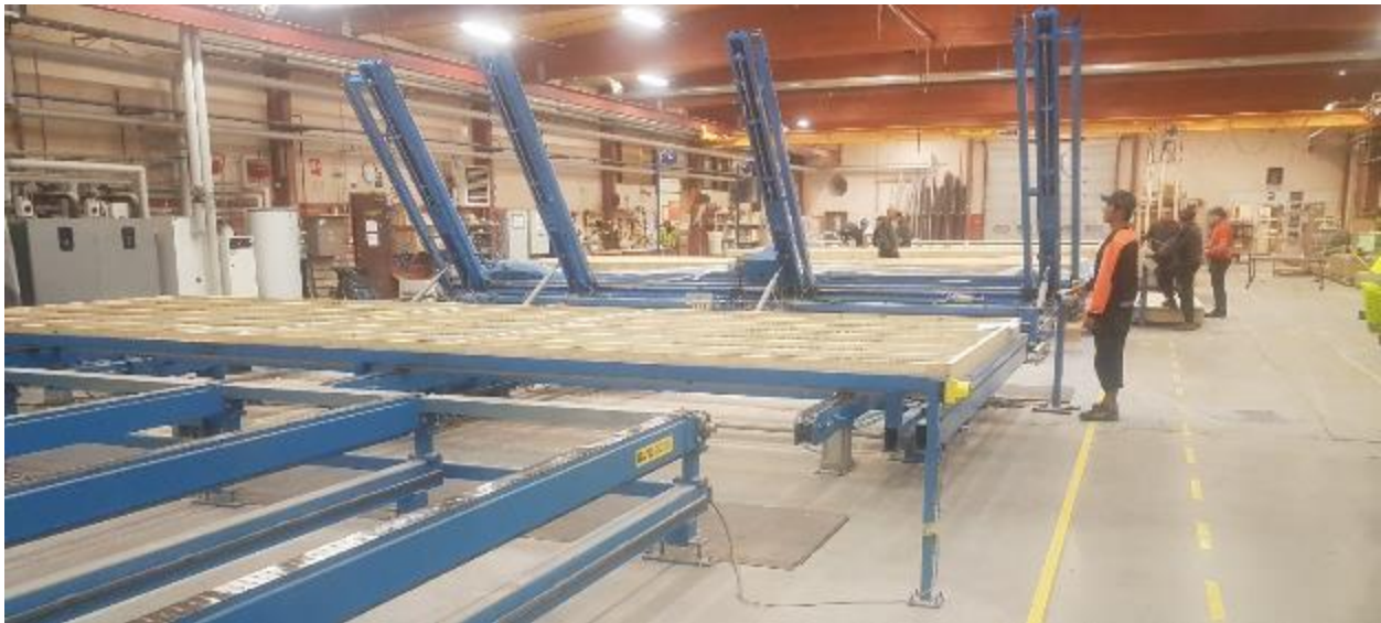
Butterfly table to flip over component allowing the finishing of both sides in Sweden (Photo: G. Wimmers)
